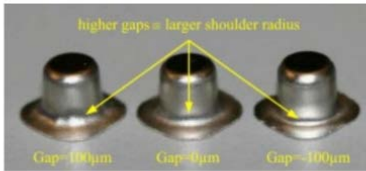
Figure 4: Cups formed with different initial gaps [12]
